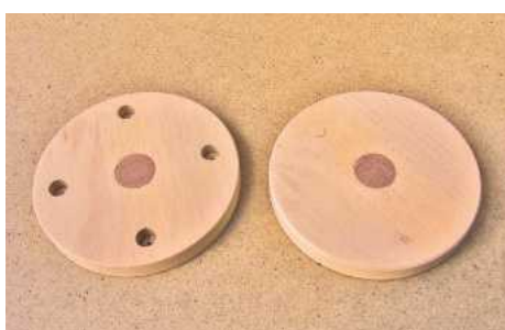
▲ Pic.4 Turn the wheels round; chamfer and polish the edges before drilling four holes in each piece
